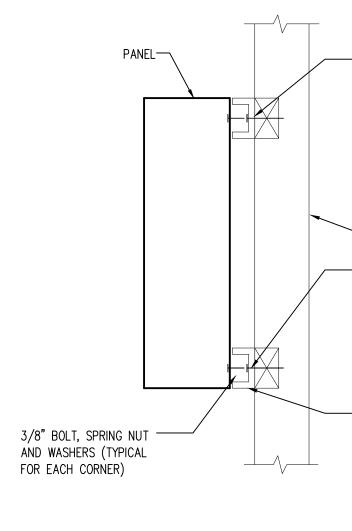
1 PANEL ON WALL DETAIL NO SCALE
